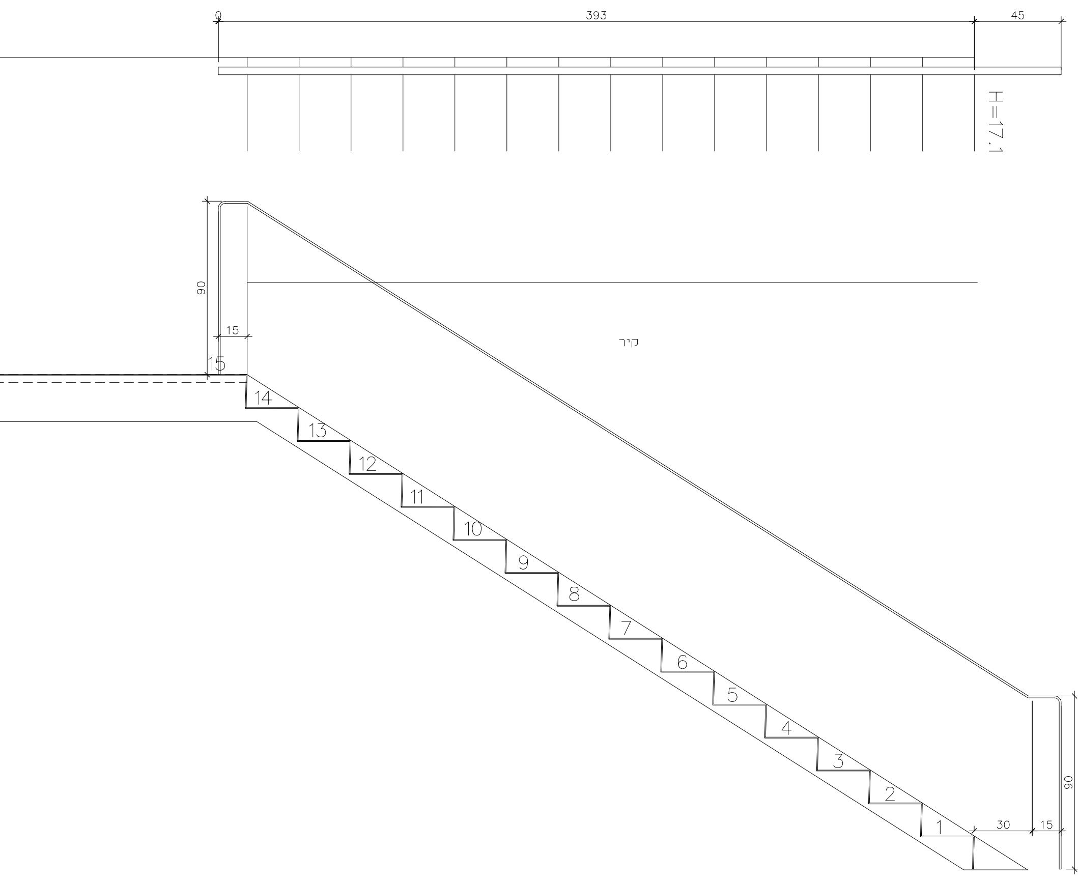
Technical drawing of a staircase section. The top part shows a horizontal view with a total width of 393 and a height H. The bottom part shows a detailed view of the stairs with 15 numbered steps and various dimensions like 90, 15, 30, 15, and 45. A label 'קיר' (wall) is present.
